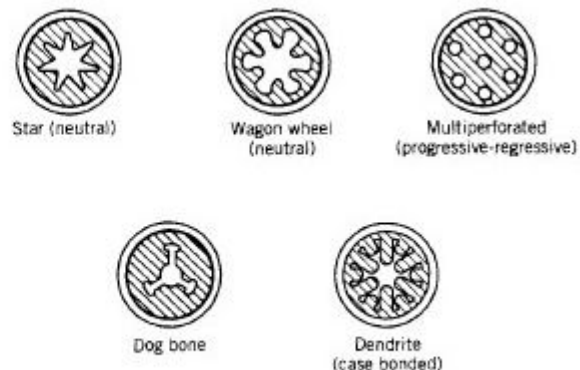
FIGURE 11-16. Simplified diagrams of several grain configurations.
